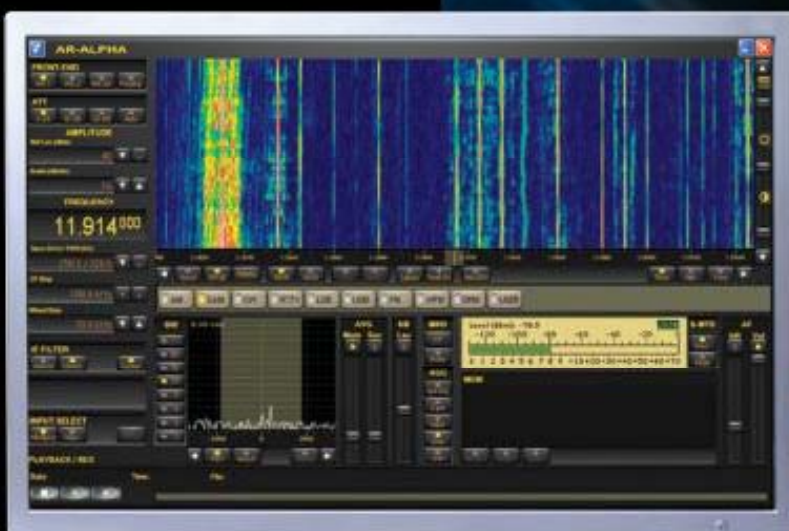
PC screen displays waterfall function to capture signal bursts
